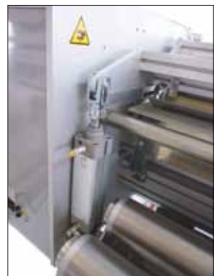
The pneumatic system makes roll loading easier
