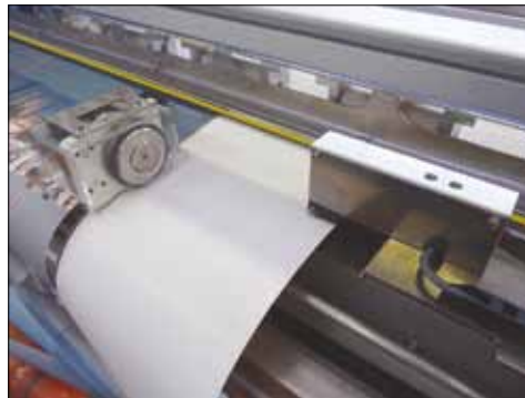
The side sensor automatically follows any roll misalignment
