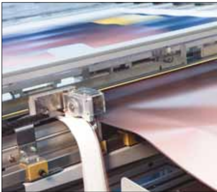
The sensor automatically follows the prints
